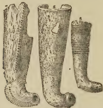
FIG. 65. Blast-pipes of smelting furnaces. 1, Silesia; 2-3, Hungary.
